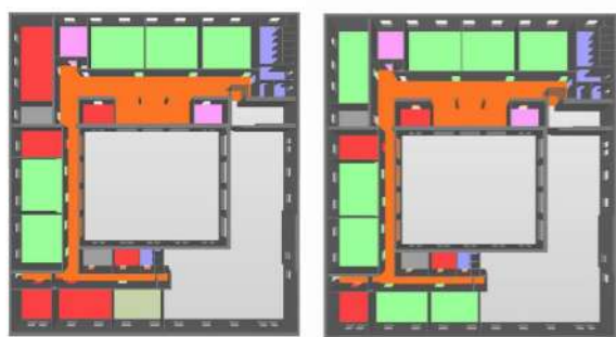
Figure 5. Change of the premises' use destination on the second floor. In green the classrooms and in red the additional educational spaces.
