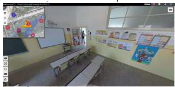
Figure 2. The building can be visited and all objects measured easily moving throughout the images acquired by the Mobile System.
