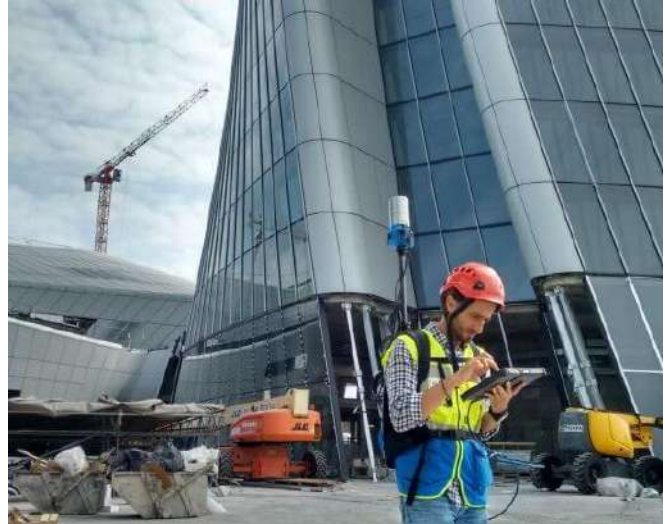
Figure 18: Italian start-up Gexcel 95 , in cooperation with the European JRC, has developed a backpack equipped with a 3D scanner for rapid mapping of indoor and outdoor sites
